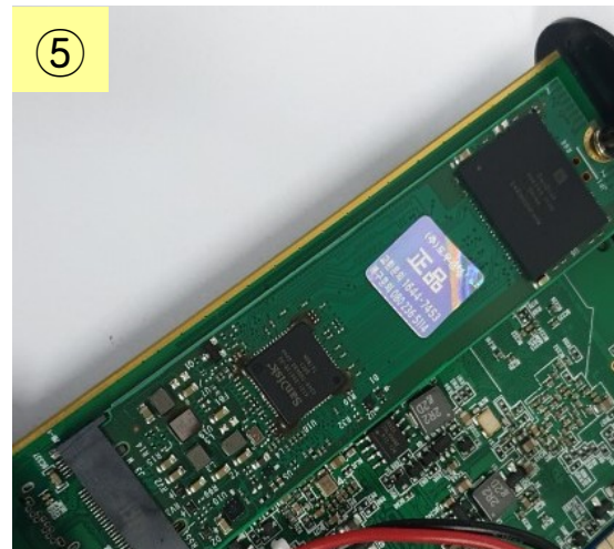
5) Fasten the M.2 screw
