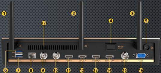
1 4G antenna **6** USB 2.0 11 HDMI – 1 Input 16 TALLY **2** 4G antenna **7** USB 3.0 12 HDMI – 2 Input 17 Cooling port **8** Gigabit Ethernet port **3** WIFI antenna 13 HDMI Display Interface 9 SDI – 1 Input 4 Switch 14 HDMI PGM Output **5** Power supply **10** SDI – 2 Input 15 SDI PGM Output
