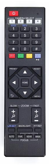
4. After changing the address, you need to select the corresponding address in 【Camera Select】 to control the corresponding camera.
