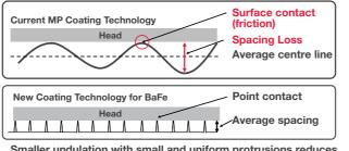
Smaller undulation with small and uniform protrusions reduces output fluctuation, resulting in less noise.
